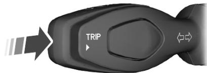
Press the end of the lever, located on the left side of the steering wheel to scroll through the displays.
