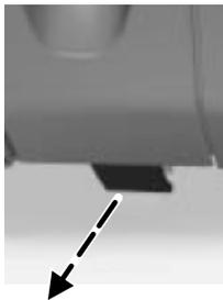
1. Inside the vehicle, pull the hood release handle located under the instrument panel.
