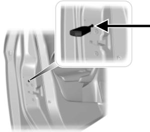
If the central locking function fails to operate, the doors can be individually locked using the key in the position shown.
