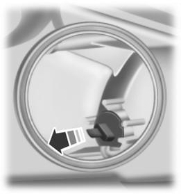
2. Turn the bulb holder counterclockwise and remove it.
