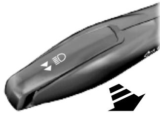
Pull the lever fully past the detent to activate. Pull the lever fully again to deactivate.
