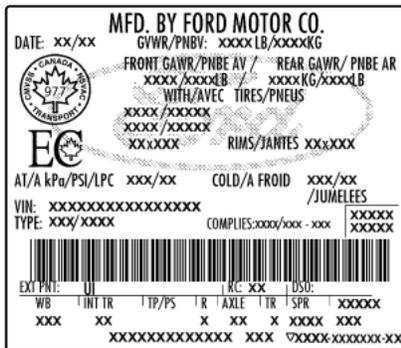
**! WARNING:** Exceeding the Safety Compliance Certification Label vehicle weight rating limits could result in substandard vehicle handling or performance, engine, transmission and/or structural damage, serious damage to the vehicle, loss of control and personal injury.
