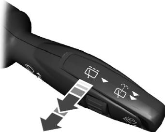
Pull the lever past the intermittent position to operate the washers.
