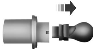
3. Reverse the procedure to install the new bulb.
