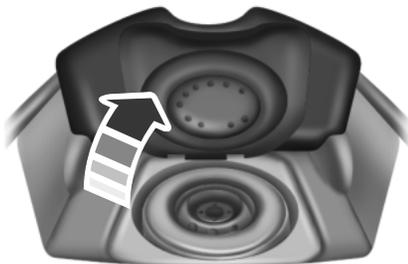
3. Remove the spare tire and jack by turning their tie-down bolts counterclockwise. The lug wrench is located in a bag next to, or on top of, the spare tire.
