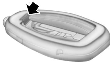
3. Twist a flat object in the position shown to separate the two halves of the transmitter.
