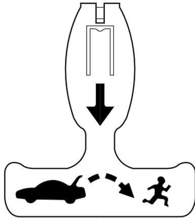
The handle is located inside the luggage compartment either on the luggage compartment door (lid) or near the tail lamps. It is composed of a material that will glow for hours in darkness following brief exposure to ambient light.
