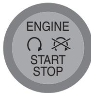
To switch the ignition on, press the start button. It is located on the right side of the steering column. All electrical circuits and accessories are operational, and warning lamps and indicators illuminate.
