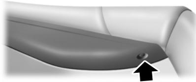
2. Using a screwdriver (or similar tool), carefully pry off and remove the passenger side console cover to expose the inside of the shifter assembly.
