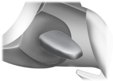
1. Locate the key backup slot on the steering column.
