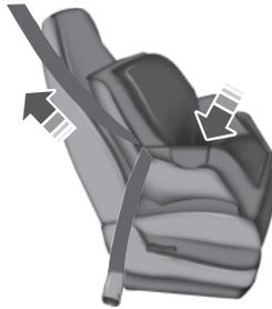
8. Remove remaining slack from the belt. Force the seat down with extra weight, for example, by pressing down or kneeling on the child restraint while pulling up on the shoulder belt in order to force slack from the belt.
