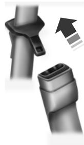
2. To unfasten, press the release button and remove the tongue from the buckle.
