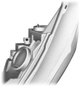
4. Locate the vertical adjuster on each headlamp. Using a Phillips #2 or 13 millimeter wrench/socket screwdriver, turn the adjuster either clockwise or counterclockwise in order to adjust the vertical aim of the headlamp. The horizontal edge of the brighter light should touch the horizontal reference line.
