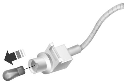
3. Reverse the procedure to install the new bulb.
