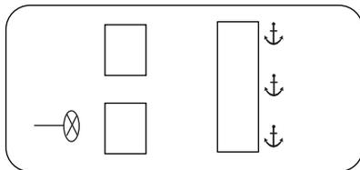
The tether strap anchors in your vehicle are in the following positions (shown from top view):
