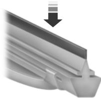
Run the tip of your fingers over the edge of the blade to check for roughness.
