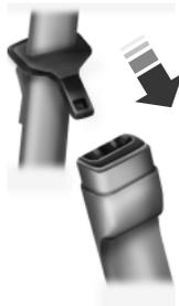
4. Insert the belt tongue into the proper buckle (the buckle closest to the direction the tongue is coming from) for that seating position until you hear a snap and feel the latch engage. Make sure the tongue is latched securely by pulling on it.
