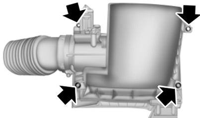
1. Remove the four screws that secure the air filter housing cover.
