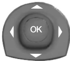
Press the up and down arrow buttons to scroll through and highlight the options within a menu.
