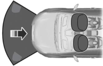
The driver and front passenger airbags will deploy during significant frontal and near-frontal crashes.
