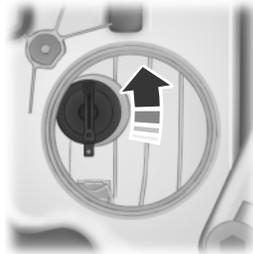
2. Turn the bulb holder counterclockwise and remove it
