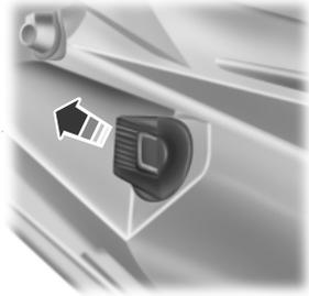
2. Remove the bulb from the bulb holder.
