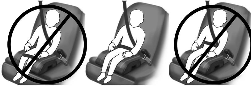
If the booster seat slides on the vehicle seat upon which it is being used, placing a rubberized mesh sold as shelf or carpet liner under the booster seat may improve this condition. Do not introduce any item thicker than this under the booster seat. Check with the booster seat manufacturer's instructions.
