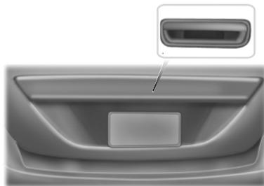
Press the exterior release button above the license plate.
