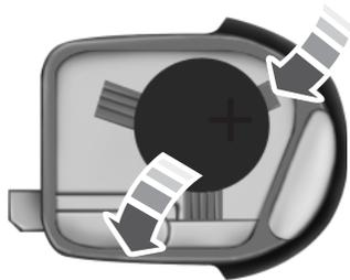
3. Carefully pry out the battery with a flat object. Be careful not to touch the battery contacts or the printed circuit board with the flat object.
