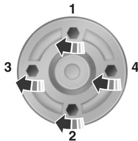
11. Remove the jack and fully tighten the lug nuts in the order shown. See *Wheel Lug Nut Torque Specifications* in this chapter for the proper lug nut torque specification.
