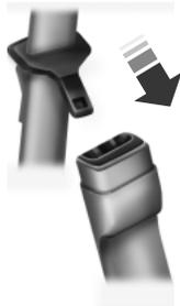
1. Insert the belt tongue into the proper buckle (the buckle closest to the direction the tongue is coming from) until you hear a snap and feel it latch. Make sure the tongue is securely fastened in the buckle.
