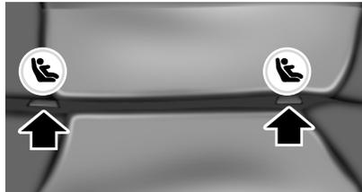
The LATCH anchors are located at the rear section of the rear seat between the cushion and seat back below the symbols as shown. Follow the child seat manufacturer's instructions to properly install a child seat with LATCH attachments.
