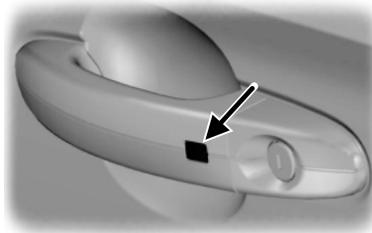
Press the sensor on the door handle to lock or unlock your vehicle.
