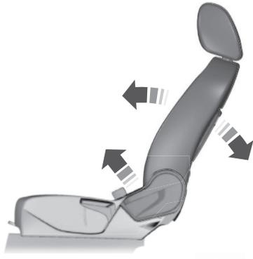
**!** **WARNING:** Before returning the seat back to its original position, make sure that cargo or any objects are not trapped behind the seat back. After returning the seat back to its original position, pull on the seat back to ensure that it has fully latched. An unlatched seat may become dangerous in the event of a sudden stop or collision.
