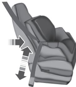
10. Before placing the child in the seat, forcibly move the seat forward and back to make sure the seat is securely held in place.
