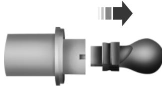
4. Reverse the procedure to install the new bulb.
