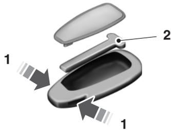
1. Press and hold the push buttons on the edges of the transmitter to release the cover. Carefully remove the cover.
