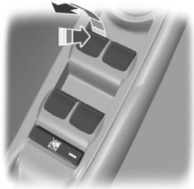
Press the switch to open the window.
