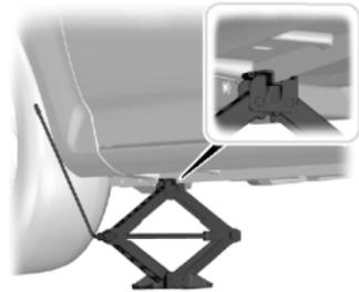
7. Position the jack in the indentions on the sill next to the tire you are changing. Turn the jack handle clockwise until the tire is off the ground.
