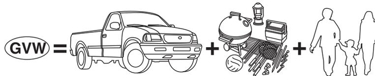
**GVW (Gross Vehicle Weight)** – is the Vehicle Curb Weight + cargo + passengers.
