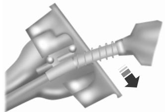
3. Slowly insert the fuel filler nozzle fully into the fuel system, and leave the nozzle fully inserted to open both doors until you are done pumping. Hold handle higher during insertion for easier access.
