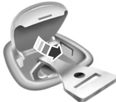
4. Clip the tether strap to the anchor as shown.
