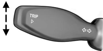
**Note:** When changing lanes, the turn signal indicator can be programmed to flash either one or three times when the stalk is tapped. See *Multifunction display* in the *Instrument cluster* section for more information.
