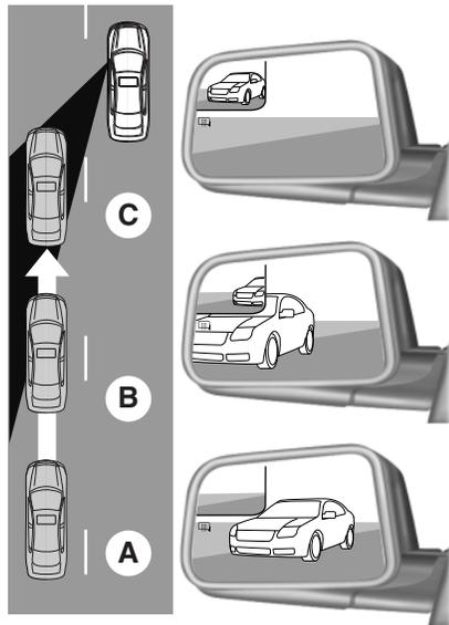
The image of the approaching vehicle is small and near the inboard edge of the main mirror when it is at a distance. The image becomes larger and begins to move outboard across the main mirror as the vehicle approaches (A). The image will transition from the main mirror and begin to appear in the blind spot mirror as the vehicle approaches (B). The vehicle will transition to your peripheral field of view as it leaves the blind spot mirror (C).
