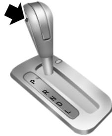
Pressing the transmission control switch on the side of the gearshift lever activates overdrive cancel and grade assist.
