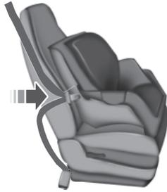
3. While holding the shoulder and lap belt portions together, route the tongue through the child seat according to the child seat manufacturer's instructions. Be sure the belt webbing is not twisted.
