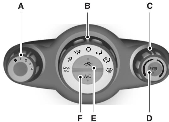
**A. Fan speed control:** Controls the volume of air circulated in your vehicle. Adjust to select the desired fan speed or switch off. If you switch the fan off, the windshield may fog up.
