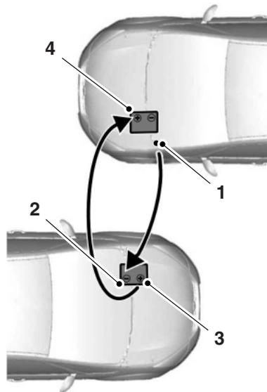
1. Remove the jumper cable from the ground metal surface.
