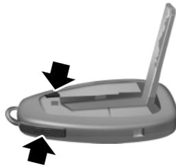
The key also contains a removable mechanical key blade that can be used to unlock the driver door. To release the mechanical key blade, press the release buttons on the edge of the transmitter and remove the key blade.
