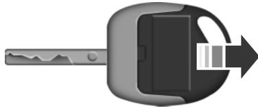
1. Carefully insert a flat object, such as a screwdriver, into the recess on the back of the key and remove the key blade.
