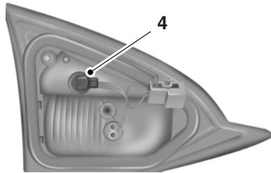
4. Turn the bulb holder counterclockwise and remove it.
