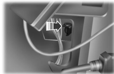
3. Locate the brake shift interlock lever on the passenger side of the shifter assembly.
