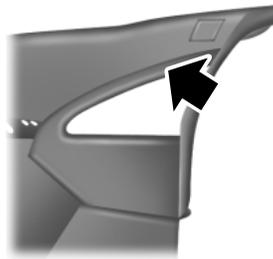
3. Carefully pull the outer upper corner of the lamp assembly to get it out of the deck lid.
