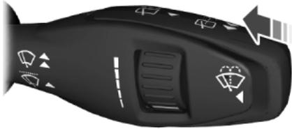
The washer will spray for as long as the lever is pressed in. After you release the lever, the wipers will operate for a short time.
