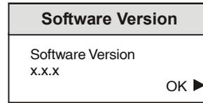
Selecting this item reveals a display showing the version of the software fitted in the module. Select OK to return to the Status Menu.
