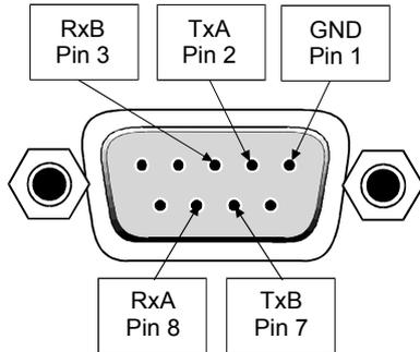
N.B. Connector is a socket, viewed from mating face. Equivalently, this is a plug, viewed from the rear, cable face.
