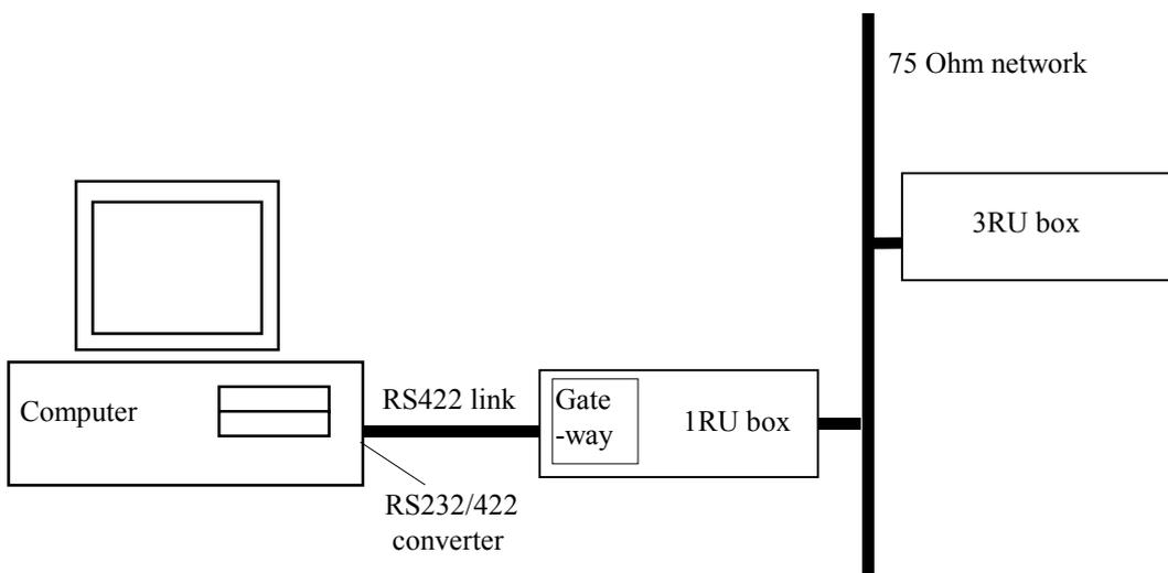
Connect the RS232/RS422 converter to COM1 or COM2 of the PC and connect this via RS422 cable to the 9 pin 'D' on the IQ modular unit. This interface is specifically designed for third party connections into the system. This allows PC's or any other serial device access to any of the units within the system. Every active 1RU or 3RU box has one of these ports.
