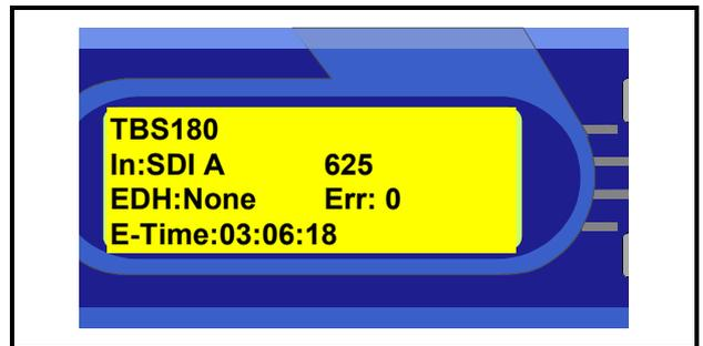
When selected the information area will display the number of errors from the time the function was enabled. The elapsed time in hours, minutes and seconds is also displayed. Meanings are as follows:
