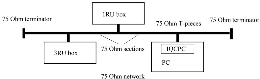
Each unit is physically joined via a T-piece connector. Each T-piece is connected by 75 Ohm co-ax cable to create a section. Each section of cable can be up to 400m. Each end of the network is terminated by a 75 Ohm terminator.
