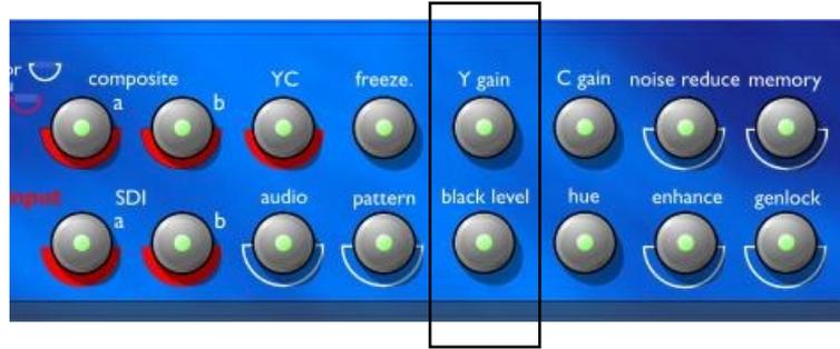
1. Restart the front panel by holding down the **Y Gain** and **Black Level** buttons together.
