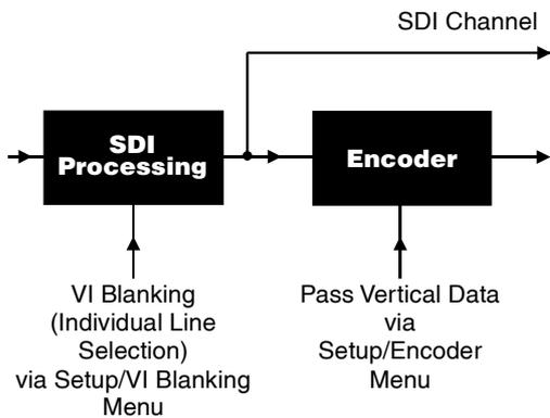
When selected input vertical data is passed on a line-by-line basis (as selected by the VBI function) into the analog signals. When not selected the vertical blanking in the analog outputs are blanked without effecting the SDI channel.
