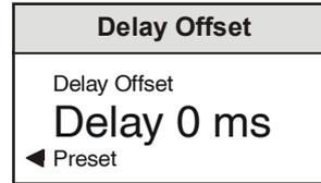
The range of adjustment is from -40 ms to +160 ms in steps of 1 ms.
