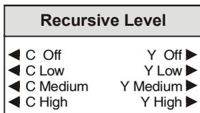
The range of adjustment is off, low, medium and high. Defaults settings are C Medium and Y Medium.
