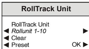
To edit the text the right ▶ and left ◀ buttons adjacent to the upper text line in the menu should be used to select the position in the text and the spinwheel used to select the character.
