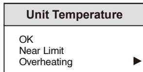
The internal temperature of the unit is continuously monitored. This item will display one of the above messages with the following meanings:
