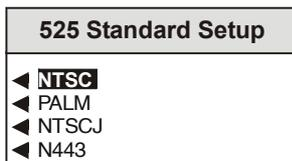
This allows the 525-line composite standard to be selected when operating in the 525-line output standard.
