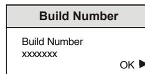
This will indicate the factory build number. This number defines all parameters of the unit (software versions, build level etc.) for identification purposes. Select OK to return to the Status Menu.
