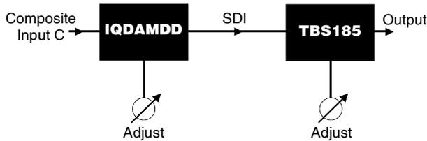
As illustrated above the Composite C signal is processed by both the IQDAMDD and the TBS185. This allows adjustments to be made by both units.
