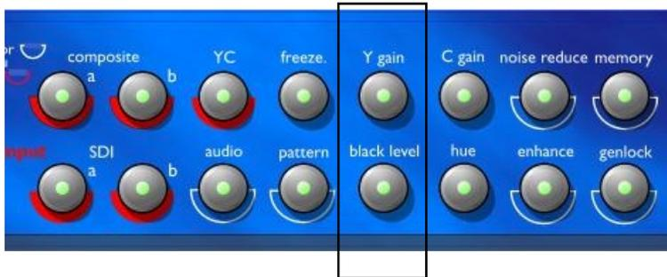
3. Restart the front panel by holding down the **Y Gain** and **Black Level** buttons together.
