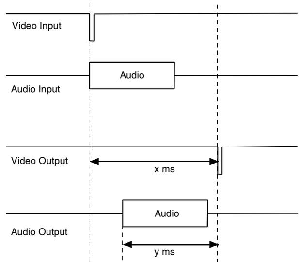
In the above diagram, the delay through the TBS180/185 is x ms. The timing of the audio output is set using the delay offset control. A negative audio delay will advance the audio by up to -x ms. The delay offset in the above diagram is -y ms.
