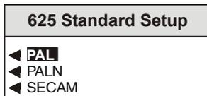
This allows the 625-line composite standard to be selected when operating in the 625-line output standard.
