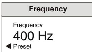
The range of adjustment is from 100 Hz to 10 000 Hz in steps of 100 Hz.
