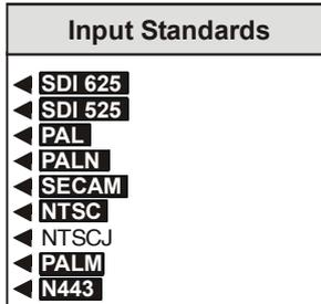
In the example above it will auto detect all standards except NTSCJ. Any number (one or more) of standards may be selected. For example, in a given situation where it is known that only PAL and NTSC input signals are expected, only the PAL and NTSC standards should be checked.
