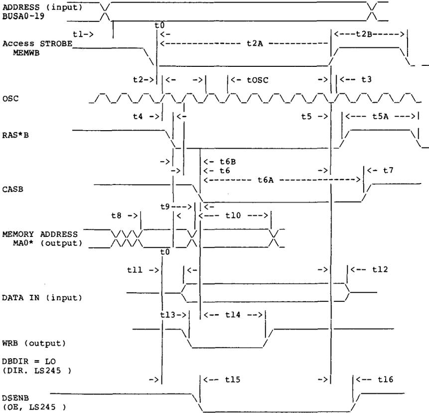
Figure 2. MEMORY TIMING PARAMETERS, WRITE
