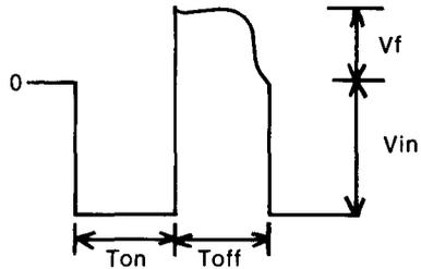
Collector Voltage Waveform
