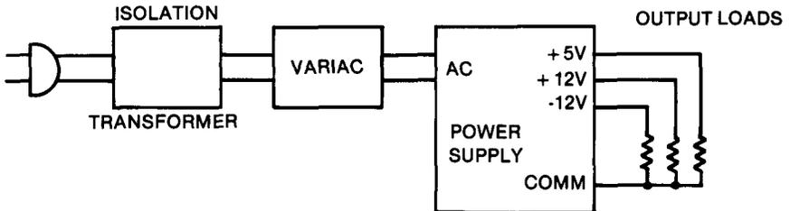
Figure 1 Test Setup
