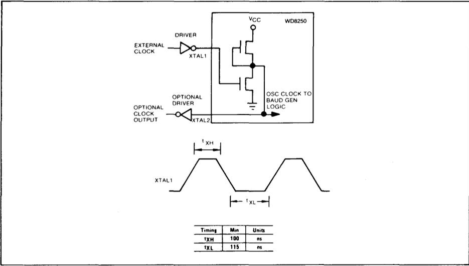
FIGURE 3. EXTERNAL CLOCK INPUT (3.1 MHz MAX.)
