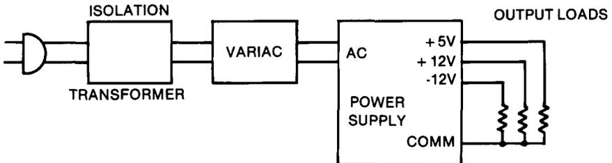
Figure 1 Test Setup
