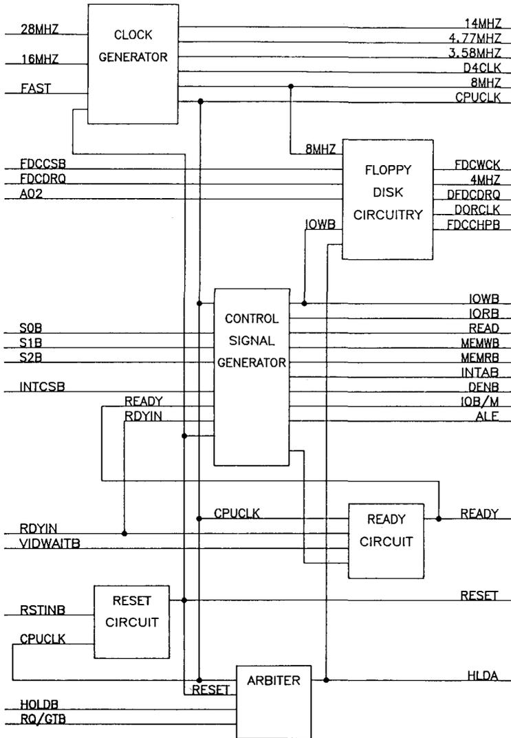
Figure 5. Timing Control Generator Block Diagram
