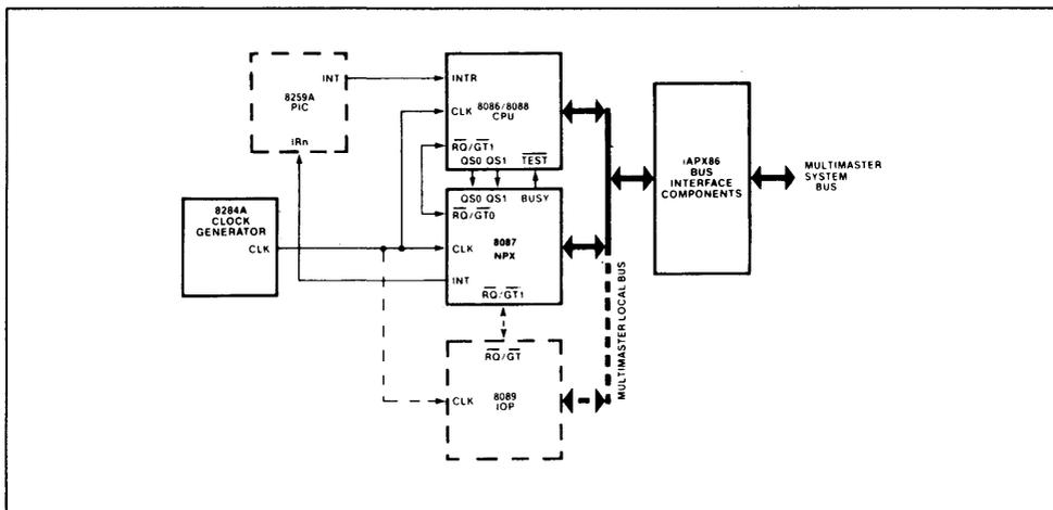
Figure 5. iAPX 186/20, 188/20 System Configuration
