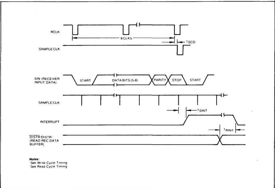
FIGURE 8. RECEIVER TIMING
