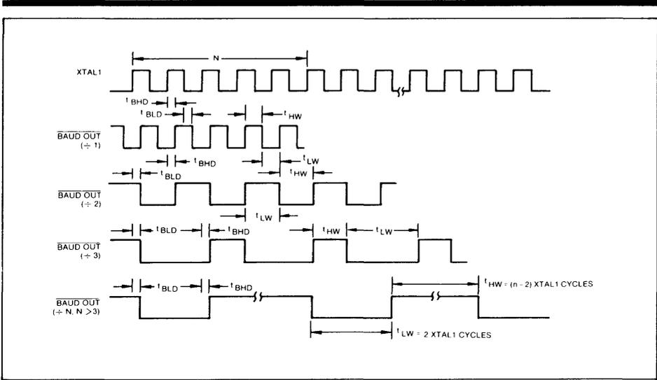
FIGURE 7. BAUDOUT TIMING
