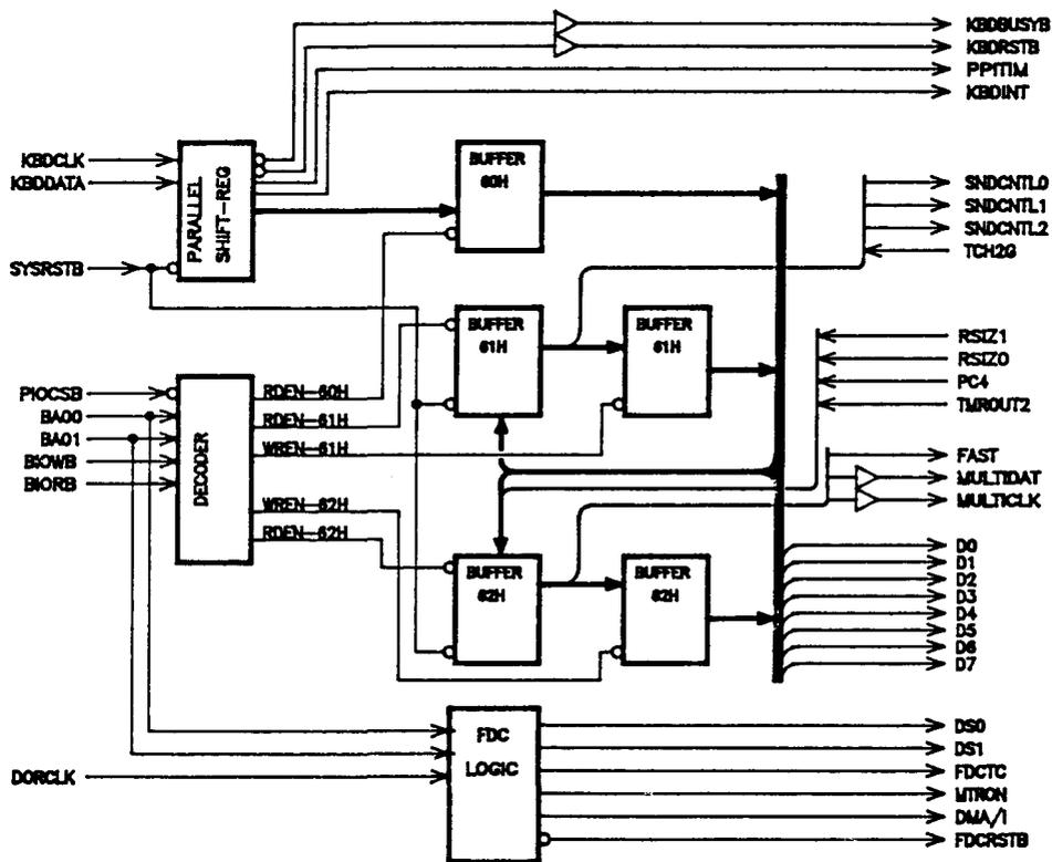
Figure 9. Keyboard Interface Block Diagram
