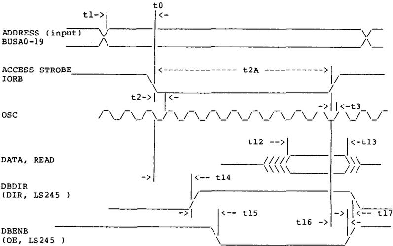
Figure 3. I/O CHIP SELECT PARAMETERS, READ
