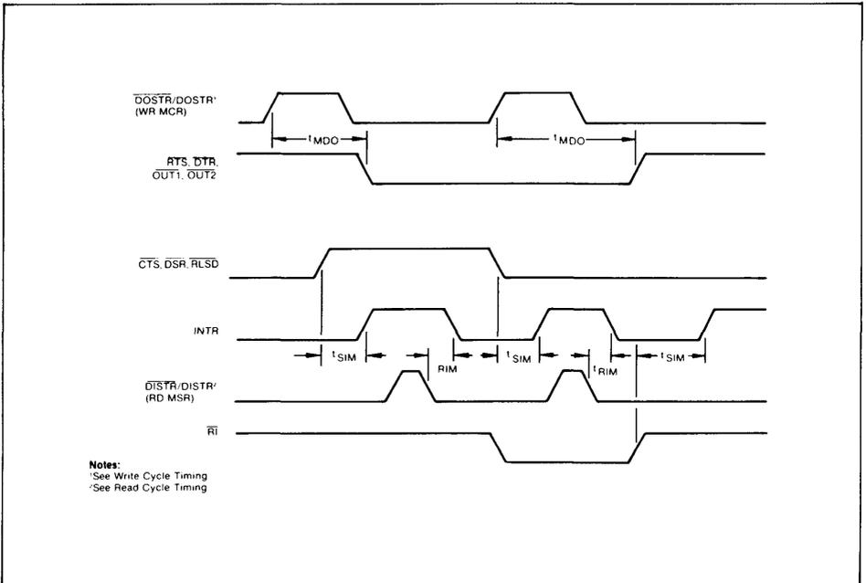
FIGURE 10. MODEM CONTROLS TIMING
