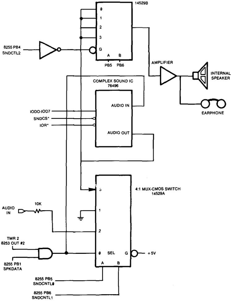
Figure 8. Sound Functional Block Diagram
