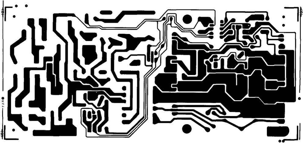
Power Supply PCB - Component Side
