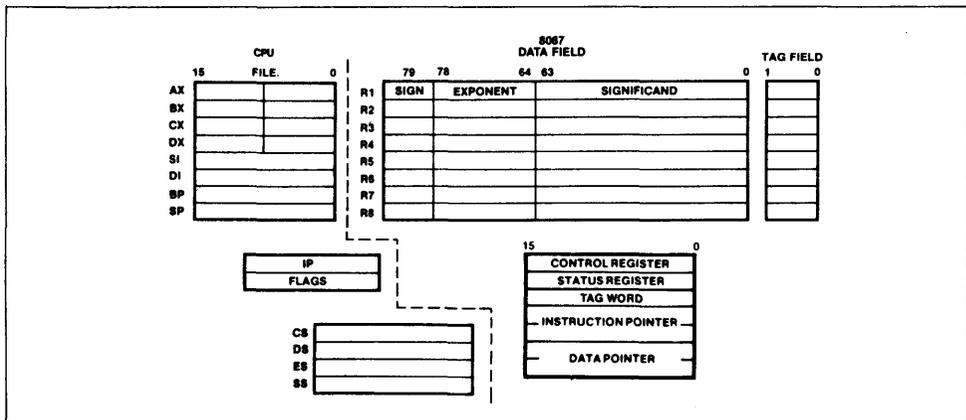
Figure 3. CPU+8087 Architecture
