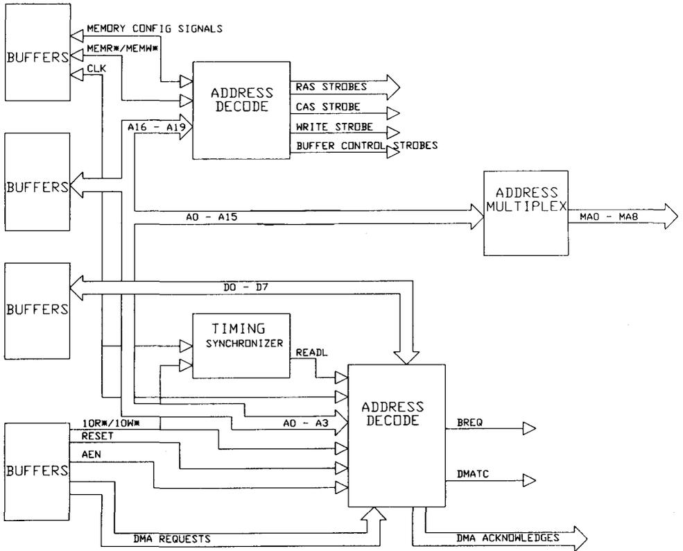
Figure 7. DMA/Memory Controller Chip Block Diagram
