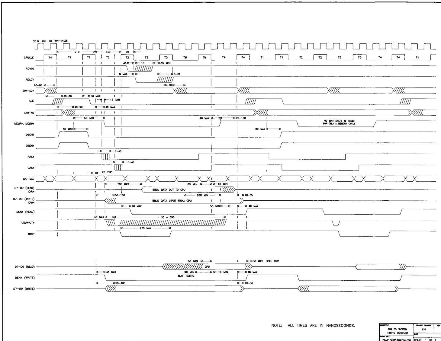
Figure 4. Tan to System Timing
