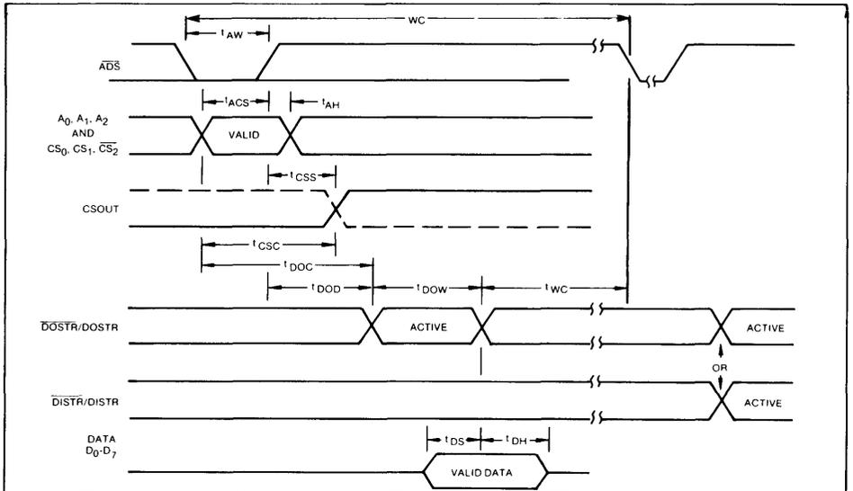
FIGURE 6. WRITE CYCLE TIMING
