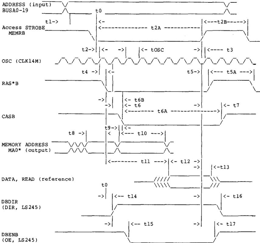
Figure 1. MEMORY TIMING PARAMETERS, READ
