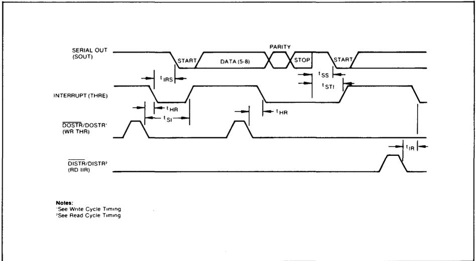
FIGURE 9. TRANSMITTER TIMING
