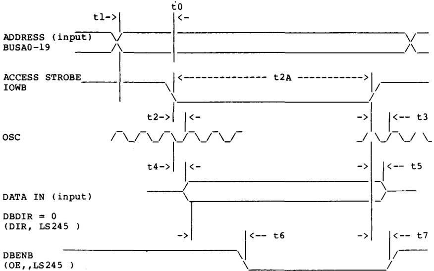
Figure 4. I/O CHIP SELECT PARAMETERS, WRITE
