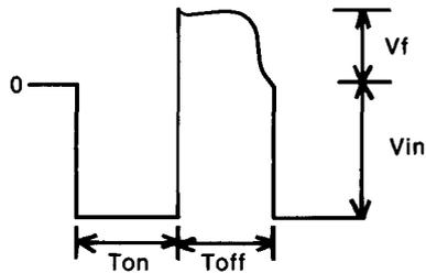
Collector Voltage Waveform
