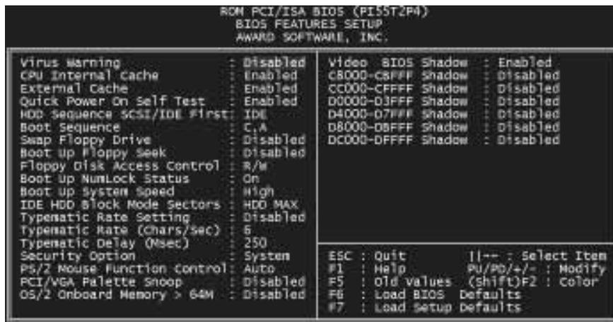
A section at the lower right of the screen displays the control keys you can use. Take note of these keys and their respective uses. If you need information on a particular entry, highlight it and then press the <F1> key. A pop-up help menu will appear to provide you with the information you need. To load the last set values, press the <F5> key. <F6> and <F7> load the BIOS default values and Setup default values, respectively.
