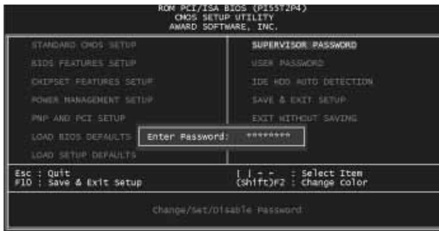
To implement the password protection, specify in the “Security Option” field of the BIOS Features Setup screen when the system will prompt for the password. If you want to disable either password, press the <Enter> key instead of entering a new password when the “Enter Password” prompt appears. A message confirms the password has been disabled.
