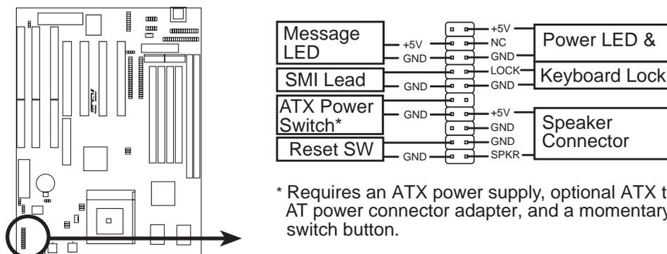
\* Requires an ATX power supply, optional ATX to AT power connector adapter, and a momentary switch button.
