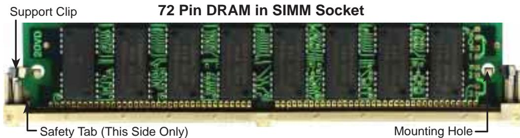
To release the memory module, push both support clips outward and rock the module out of the support clips.
