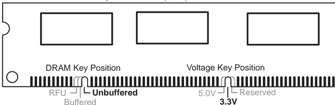
The notch on the DIMM module will shift between left, center, or right to identify the type and also to prevent the wrong type of DIMM to be inserted into the DIMM socket on the motherboard. Four clock signals are supported on this motherboard. You must ask your retailer for the specifications before purchasing memory modules.
