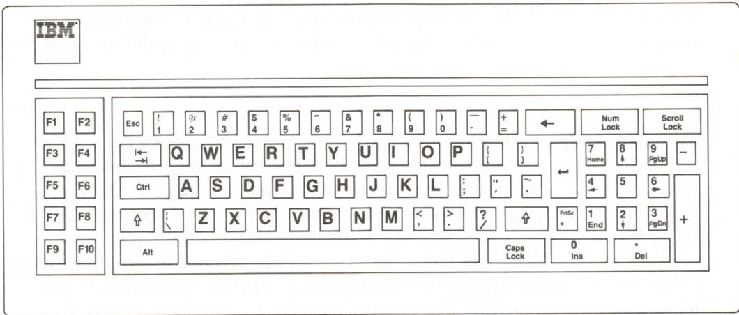
Figure 12-2. The PCjr and the PC/XT keyboards
