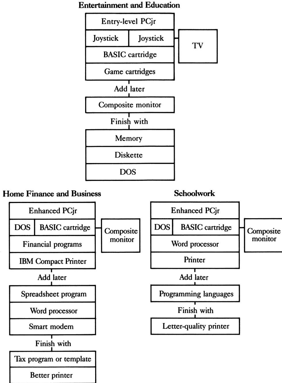
Figure 2-8. Equipment and software for the three main uses for a PCjr
