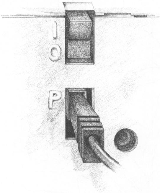
Figure 3-1. How the transformer plugs into the PCjr
