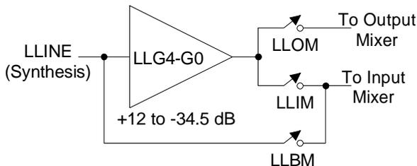
When IFM=1 (X4 or Global Config. byte) and FMRM=1 (X4), FM remapping is enabled. When WTEN=1 (C8 or Global Config. byte) and WTRMD=0 (X4), Wavetable remapping is enabled. If either synthesizer remap is enabled, left LINE analog volume is controlled through X0. With remapping the bit definitions are:
