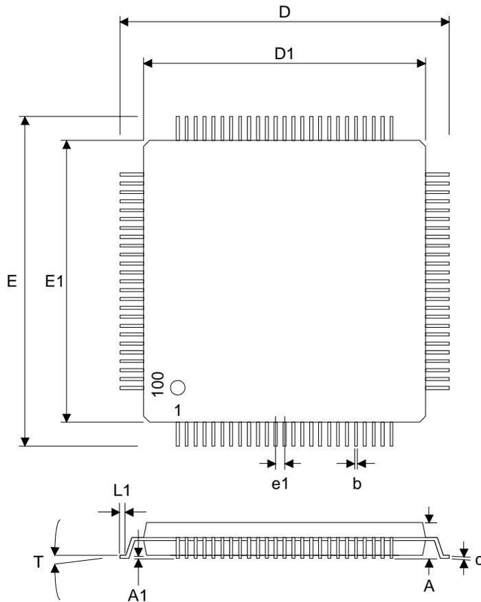
**100-pin TQFP - Package Code 'Q'**
