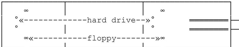
5. Slide the drive into the drive tower until the rails lock into place.
