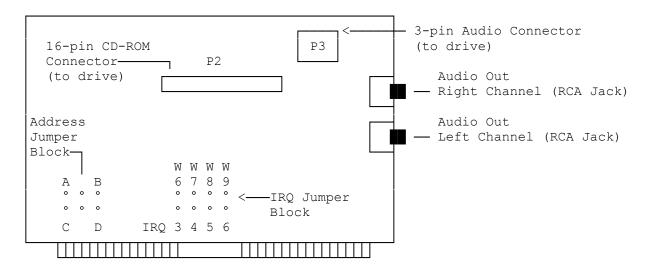
The adapter interface card lets the CD-ROM drive and your computer communicate with each other. Before you install the adapter interface card, you must select its port address and IRQ channel settings.
