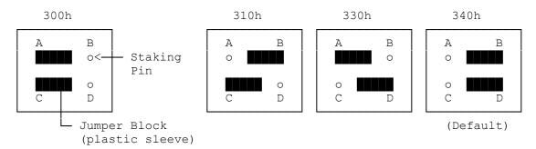
The above illustrations show the adapter interface card port address settings. (The default port address is, 340h. The letter "h" indicates
