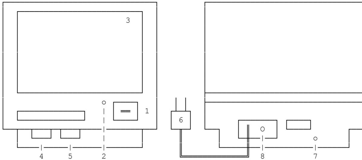
1. POWER ON/OFF SWITCH. Press to turn the VM-1's power ON. Press again to turn the power OFF.
