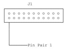
The host adapter will initiate SCSI synchronous negotiation during initialization of after a SCSI reset if this jumper is installed. If the jumper is not installed, the host adapter will still support synchronous SCSI transfers, but the target must initiate the negotiation. Default is jumper removed, synchronous negotiation initiation disabled.
