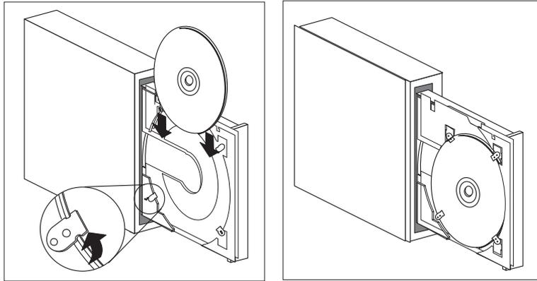
4. Close the tray by pressing the Eject/Load button, or by gently pushing the tray forward. When the tray is closed, the indicator light on the front of the drive will activate to indicate that the drive is in use.
