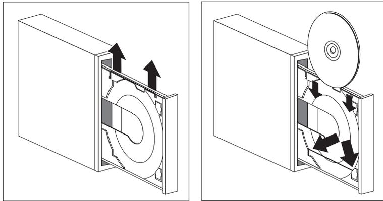
6. Because of the spring-tab, you can lift the support wire when you insert a CD and let it hold the CD in place. Close the tray by pressing the Eject/Load button, or by gently pushing the tray forward. When the tray is closed, the indicator light on the front of the drive will activate to indicate that the drive is in use.
