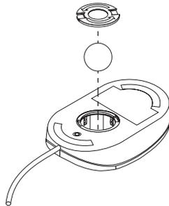
4. Turn the mouse right-side up, and the retainer and ball will drop out.
